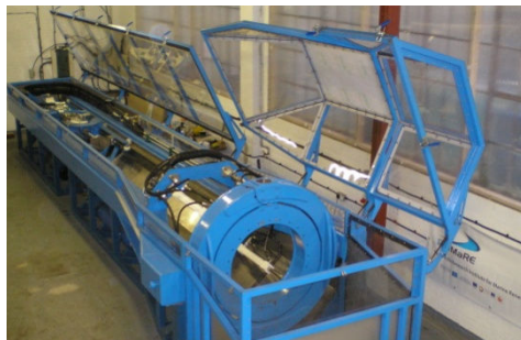
Figure 1: Dynamic Marine Component Test rig (DMaC)
